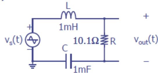
$$\text{Soln.: } V_{out}(s) = \frac{R}{sL + R + \frac{1}{sC}} V_{in}(s) = \frac{sRC}{s^2LC + sRC + 1} V_{in}(s)$$
